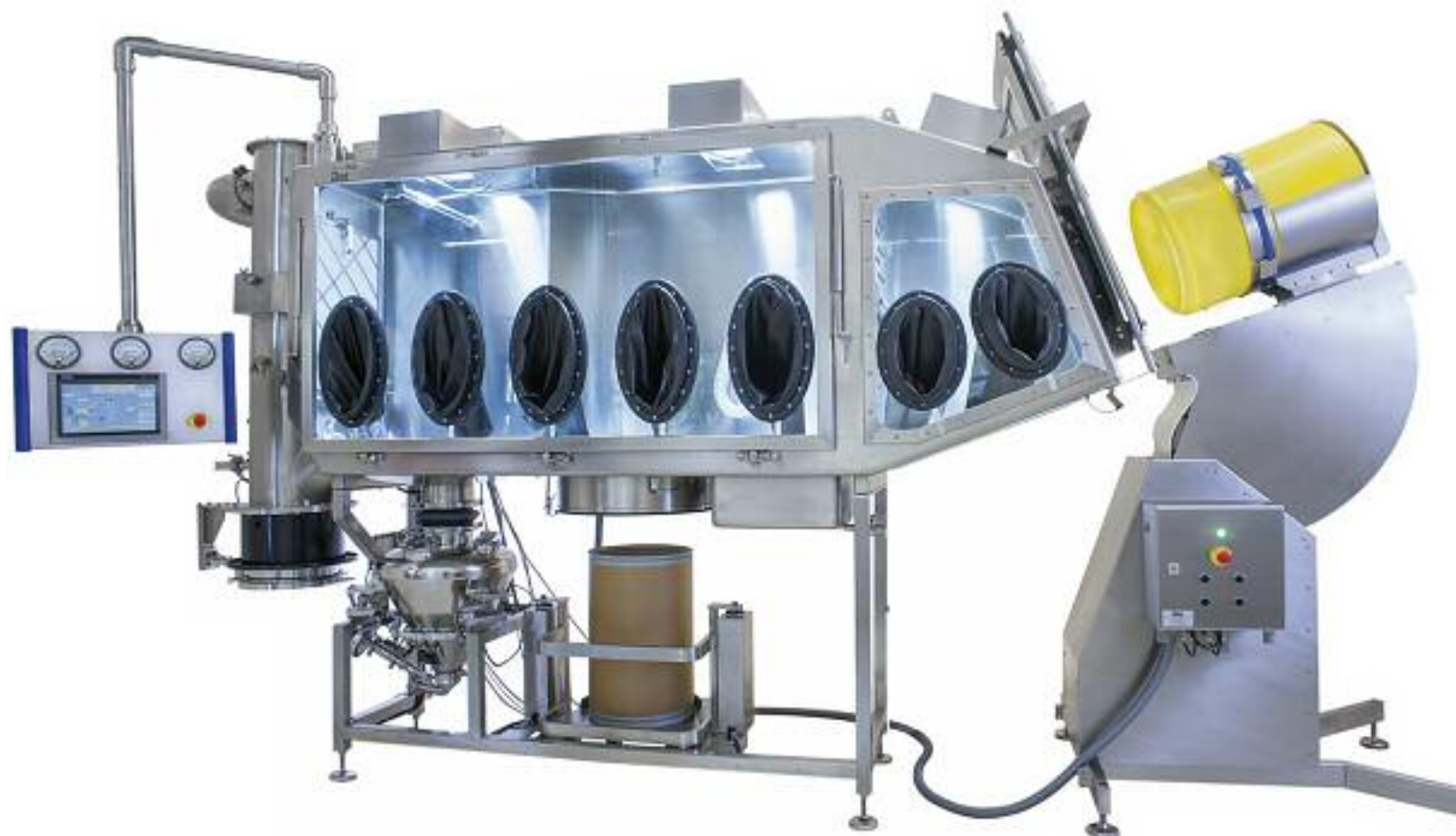
Isocharge – contained dispensing and reactor/equipment charging in combination with the PTS Powder Transfer System®
